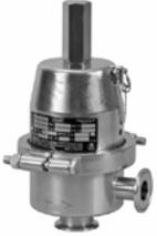
Fisher™ Type SR5 regulator is a compact, large capacity, self-operated pressure reducing regulator. It is designed for use in applications where a sanitary design is essential, such as pharmaceutical, biotech, or food and beverage industries. The unit is available in NPS 1/2 through 3 / DN 15 through 80 sizes with end connections that will match up to Tri-Clamp sanitary fittings. Type SR5 is suitable for use in steam, liquid or gas service.
