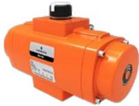
The Bettis™ RPE-series is a rack & pinion actuator, available in 12 sizes as spring return or double acting models. The actuators have a tough and reliable design and are intended to operate quarter turn valves or any other quarter turn application. The Bettis RPE-series comes with coated body and endcaps, has a special high corrosion resistant aluminum pinion design and has stainless steel fasteners, resulting in a long lasting durable actuator design.
