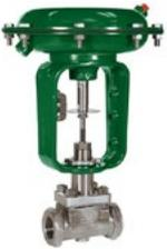
The Baumann™ 24000S control valve is versatile, pneumatic, and may be used for the control of pressure, temperature, level, and flow. The CF8M stainless steel valve body will withstand mildly corrosive fluids, yet is economical enough to use in applications where carbon steel is normally specified.
