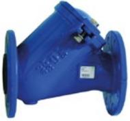
VAG KRV® is a resilient-seated non-return valve with sinking ball and free flow passage for minimum friction loss. Especially suitable for use in polluted media as the shape of the valve prevents the build-up of dirt. Highly maintenance-friendly due to the large clean-out hole. Suitable for use in waste-water applications, in power plants and in industry.
