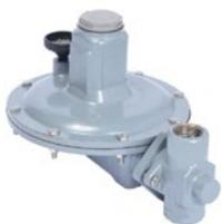
The Fisher™ T205 Series tank blanketing regulator is a direct operated and spring-loaded regulator. The T205 Series maintains a slightly positive pressure to prevent a stored liquid from vaporizing into the atmosphere, reduces liquid combustibility, and prevents oxidation or contamination of the product by reducing its exposure to air.
