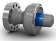
A complete line of Fisher inline diffusers provide optimum noise attenuation where valves can contribute substantial noise. When installed, the total pressure drop of the system is divided across the valve and diffuser. This enables the valve to operate at a lower pressure drop ratio, thereby lowering the noise level generated from the process flowing through the control valve. Options include: the 6010 with integral outlet head, the 6011 pipe style, and the Whisper Disk.
