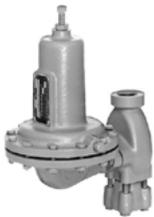
Fisher™ Type 630 Big Joe™ regulators are direct operated, spring-loaded, pressure reducing regulators available in NPS 1 & 2 / DN 25 & 50 body sizes designed for maximum inlet pressures to 1500 psi/103 bar and outlet pressures from 3-500 psi/0.21-34.5 bar. Type 630 can be used with natural gas, air, or a variety of other gases for such applications as first-stage farm-tap or high-pressure industrial regulators. They can be converted to a relief valve in the field.
