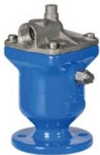
VAG DUOJET® Automatic Air Valve. High-capacity, single-chamber air valve with triple function for venting and releasing air in pipelines as well as for releasing air during operation. Corrosion-proof due to stainless steel inner parts and float made of plastic. Safe and reliable operation even at high air-release velocities of up to sonic speed. Suitable for use in water treatment, water distribution, in dams, power plants and in industry.
