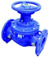
Externally controlled control valve for the regulation of the pressure and flow rate in service areas with external power supply. The control characteristic can be adapted to the operating conditions by means of a finely slotted cylinder serving as control insert. Suitable for use in water treatment, water distribution, in power plants, in industry and in pressure management. VAG DURA is also available with manual gearbox and electrical actuator.
