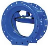
VAG SKR® Metallic-sealing non-return valve with slanted seat for reducing the closing time and with specially shaped disk that supports the opening movement. Also available with internal damping unit for the reduction of pressure surges. The prerequisite for trouble-free operation is a minimum flow velocity of 1.5 m/s in the customer's plant. Suitable for use in water treatment applications, water distribution, in pretreated sewage, in power plants and in industry.
