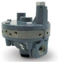
Fisher™ VBL volume booster is used in conjunction with a positioner on a throttling control valve to increase stroking speed. The booster incorporates fixed deadband, soft seat construction, and an integral bypass restriction to eliminate positioner saturation problems. The volume booster delivers high volume output for fast stroking when large, rapid input signal changes occur.
