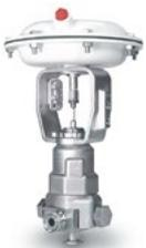
The Baumann™ 83000 sanitary angle control valve is excellent for the control of high purity fluids or gaseous media. A low-friction force amplification mechanism, comprised of a roller bearing linkage, produces high-positioning resolution suitable for direct operation from remote I/P signal converters.
