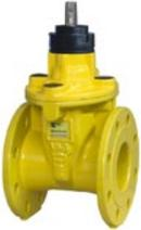
VAG EKO®plus is a resilient-seated gate valve with bolted cover connection and face-to-face length of Basic Series 14 for gas applications. Proven design with innovative improvements, such as plastic sliding caps on the wedge, guarantee low operating torques even after many years of use. Suitable for use in gas main and service pipelines as well as pressure stations and gas storage tanks
