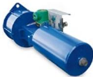
Double acting and spring return pneumatic quarter turn actuators for on-off and modulating control of valves in heavy duty service. Available for output torques to 750,000 Nm. Totally enclosed, weatherproof housing in fabricated carbon steel for maximum strength. Guide bar resists transverse loads and supports the piston rod. Hard chromium plated alloy steel material guarantees corrosion protection and minimal friction.
