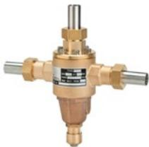
The type PBE-5 regulator is a fully automatic pressure building/economizer valve designed for cryogenic liquid systems. It is equipped with a non-adjustable/fixed set point economizer. The valve is also equipped with bullnose tube connections that incorporates a check valve to prevent backflow into the economizer. An indicating adjustment screw provides an easy field adjustment reference.
