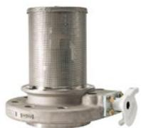
Fisher™ C404-32 flanged internal valve has gained wide field acceptance for use as primary shutoff valve, excess flow valve and back check valve. The valve can be used in conjunction with or without pumps and compressors. Because of the integral back check function of this valve, selective filling of manifold storage tanks requires the use of additional shutoff valve.
