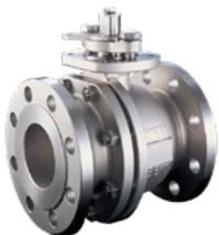
Versatile KTM Series EB1 is a high performance, next generation ball valve with bidirectional soft-seats, LOW-E fugitive emission certification, high pressure & temperature options and competitive design with cavity relieving seats.
