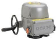
Keystone™ EPI2 series are compact, intelligent quarter-turn electric actuators for the accurate control of valves with torques from 35 to 2000 Nm / 308 to 17,700 lb.in. Separate terminal enclosure isolated from the electronics and motor compartment; only the wiring terminal is exposed during field installation. Latched-type output contacts for fully open/ fully close remote indication. Output contacts for monitor and blinker/local selector indication are also available.
