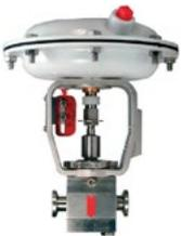
The Baumann™ 87000 control valve is excellent for throttling high purity liquid or gaseous media commonly found in the food and beverage, pharmaceutical, film, and biotechnology industries. This valve is suitable for repeated steam sterilization cycles with 2.4 bar (35 psi) maximum steam pressures.
