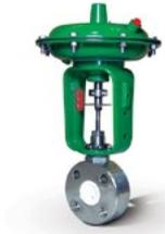
The Baumann™ 26000 valve is a unique corrosion-resistant control valve featuring a flangeless wafer valve body and powerful multi-spring diaphragm actuator. A solid corrosion-resistant R05200 Tantalum or N10276 nickel alloy valve plug and pressure-assisted PTFE seat combine for an extremely wide control range making the 26000 series ideal for pH control applications. Top entry trim provides ease of servicing and a long operating life.
