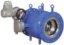
VAG RIKO® is plunger valves with either handwheel or electric actuator. Externally controlled one-piece body control valve with annular flow cross-section for the continuous regulation of high pressure differences and flow rates. Long service life as the bearings do not come into contact with the medium. Also available as own-medium controlled control valve. Suitable for use in water treatment, water distribution, in dams, power plants, industry and in pressure management.
