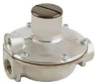
The Fisher™ 912N Series direct operated, spring-loaded regulators are used in service and industrial applications. These regulators have limited-capacity internal relief across the diaphragm to help minimize overpressure. Any outlet pressure above the start-to-discharge point of the non-adjustable relief valve spring moves the diaphragm off the relief valve seat, allowing excess pressure to bleed vent. 912N Series regulators are built to provide accurate, sensitive control.
