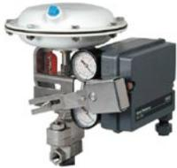
Fisher™ 3661 electro-pneumatic single-acting positioners are used with various actuators on sliding stem valves for throttling applications. These rugged positioners provide a valve position proportional to a pneumatic input or a standard millampere DC input signal received from a control device.
