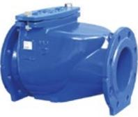
VAG RETO-STOP® is a resilient-seated, slanted-seat check valve that opens even at low differential pressures. The disk can be used on both sides, which doubles its useful life. The one-piece and completely rubber-coated disk ensures a completely free passage and reduces the adhesion of dirt particles. Suitable for both horizontal and vertical installation in water treatment plants, in water distribution, in waste-water applications, in power plants and in industry.
