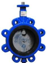
The VAG CEREX® 300-W Wafer-Type and 300-L Lug-Type Butterfly Valves are resilient-seated valves with disks made of stainless steel. 300-W for flange mounting between pipelines and 300-L for flange mounting to pipelines. With replaceable liner mounted on a vulcanised seal carrier ring, and disk with triple bearing. With NBR seal for wastewater and gas or EPDM for water. DVGW tested and registered.
