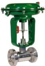
The Baumann™ 24000SB control valve is recommended for low flow, high pressure, and industrial control applications. The 24000SB valve is the ideal solution for applications that exceed the operating range of other Fisher 24000 series valves. Various end connections ranging from threaded (standard), butt weld, and flanged add versatility to this high-pressure product line. Special high nickel alloy constructions are available and round out the basic S31600/S31603 stainless steel offering.
