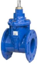
VAG EKO®plus is a resilient-seated gate valve with bolted cover connection and face-to-face length of Basic Series 14 for waste-water applications. Proven design with innovative improvements, such as plastic sliding caps on the wedge, guarantee low operating torques even after many years of use. Suitable for waste-water applications and in water-treatment plants of power plants and industry.
