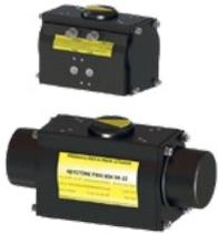
Keystone™ F89 is a pneumatic quarter-turn actuator for general purpose and hazardous area applications. The F89 is designed for simple, safe use and ultimate reliability, meeting EN15714-3 requirements and has been validated to 500,000 cycles under specified conditions.
