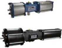
B series- Ductile iron w/ stainless steel cylinders, C series- Ductile iron w/ carbon steel cylinders Spring return and double acting actuators Quarter-turn output torques to 158200 Nm. Ductile iron housing, piston and end caps provide long life and durable, cost-effective operation. High strength alloy steel or 17-4PH stainless output shaft transmits torque without fatigue. Strong, corrosion-resistant chrome-plated steel piston rod for enduring high cycle applications.
