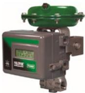
The Baumann™ 51000 control valve is optimally designed for demanding low flow, high pressure control applications often found in laboratories and pilot plants. NPS 1/4 or 1/2 valve assemblies are standard as either investment cast stainless steel or N10276 nickel alloy. Constructions with other high nickel alloys are available.
