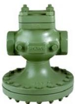
The Type E Main Valve is pilot-operated normally closed, single seat design featuring packless construction, balanced metal diaphragms and protected main spring. One or more pilot regulators are mounted to Type E Main Valve to fit with the specifications defined by the pressure regulating system. For fluid, gas and vapor applications.
