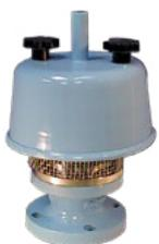
Weight or spring loaded pressure relief valves with a wide variety of material and sizing options that vent to atmosphere. The 4130A is designed to satisfy the requirements of the liquid storage industry in storage tank farms, in the petroleum and chemical sectors, in refineries and terminals.
