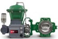
The Control-Disk™ rotary valve offers excellent throttling performance. An equal percentage flow characteristic provides an improved throttling range comparable to that of a segmented ball valve. This improved capability allows you to control closer to the target set point, regardless of process disturbances, which results in a reduction in process variability.
