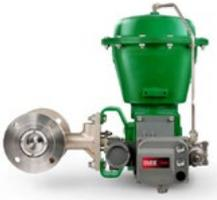
The Fisher™ CV500 valve combines the rangeability of the cammed, segmented V-notched ball, with inherent ruggedness in the heavy duty bearings, seals, and body. This combination provides a balance of erosion resistance and pressure control for gas and liquids.
