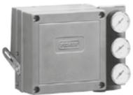
Fisher 3582™ pneumatic valve positioners are used with diaphragm-actuated, sliding stem control valve assemblies. This pneumatic valve positioner receives a pneumatic input signal from a control device and modulates the supply pressure to the control valve actuator, providing an accurate valve stem position that is proportional to the pneumatic input signal.
