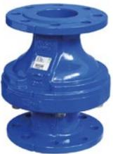
VAG TOP-STOP® Resilient-seated non-return valve with diaphragm and internal flow guide for the fast and noiseless shut-off against the return flow. Suitable for installation in any position. Due to the elastic diaphragm the valve has optimum pressure-surge damping properties. Suitable for use in water treatment applications, water distribution, in power plants and in industry
