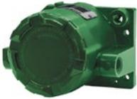
A Fisher FIELDVUE 4400 digital position transmitter senses the position of rotary or sliding-stem valves, vents, dampers, or other devices. It provides a precise non-contact feedback to indicate equipment position with a percent (%) of span plus on/off indication. The 4400 provides 4-20 mA position feedback, is SIL 2 capable, and has two 1-amp NAMUR design solid-state limit switches.
