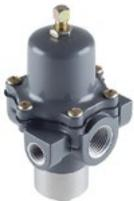
167D Series switching valves are used to deliver constant reduced pressure of gaseous fluids to pilot-operated controllers and other pneumatic instrumentation. Types 167D and 167DS are two-way switching valves. Types 167DA and 167DAS are three-way switching valves.
