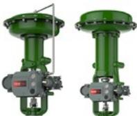
Fisher™ 657 and 667 actuators are designed to provide dependable on/off or throttling operation of control valves. These spring-opposed diaphragm actuators position the valve plug in the valve in response to varying controller or valve positioner pneumatic output signals. The 657 actuator is direct-acting, while the 667 is reverse-acting.
