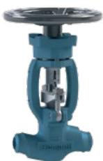
Sempell™ model VA 500 is an isolation valve for high pressure and high temperature systems. Robust valve with one-piece dye cast body, Stellite body seat, visual position indicator, non-rising stem. Simple adaption to motorization with electrical actuator. As standard with weld end connection. Flanges upon request.
