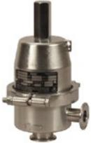
Fisher™ Type SR8 backpressure regulator is a compact, large capacity, direct operated backpressure regulator. It is designed for use in applications where a sanitary design is essential, such as pharmaceutical, biotech, or food and beverage industries. The unit is available in NPS 1/2 through 3 / DN 15 through 80 sizes with end connections that will match up to Tri-Clamp sanitary fittings. Type SR8 is suitable for use in steam, liquid or gas service.
