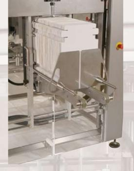
The positive drive magazine is placed at an ideal height, which makes it easy to fill up with new blanks.
