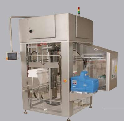
The machine is made of stainless steel. All drives and electrical parts are placed above the working area.
