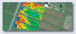
GPS-signal acquisition is an additional function of Delphin's data logger. GPS signals are received and transmitted via a serial cable to provide the location of the measurement data being acquired. Evaluation is performed via KML files and Google Earth $^{\text{TM}}$ .
