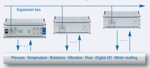
Plant and machinery that make up a process are usually located across several different sites. Data acquisition for such processes is often performed decentrally. Message hardware and ProfiSignal software are ideal for decentralized data acquisition. The systems can be locally installed and connected via Ethernet or CAN-Bus. Data storage can be performed both centrally and decentrally.
