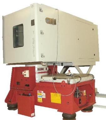
Combined climatic and vibration test
