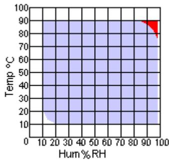
For climatic tests that require humidity and temperature ranges highlighted **in red** on the graph, a Psychrometric sensor is recommended (EP and ECP models). Please consult Aralab for help on the choice between these two models.
