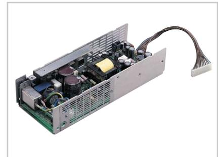
A lot of designs of power product, the insulation capability of input terminal (Primary) to output terminal (Secondary) is required to protect the damage inside component. Thus, the output terminal of Floating needs to perform Hipot test. The 19032 provides isolation test point with high voltage to let you no need to change fixture or cable by manually that performs P-S Hipot test directly after P-G Hipot test.
