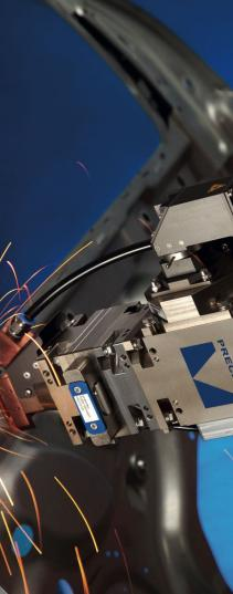
The laser welding is performed on many types of material, sometimes using pure argon or mixed, and in many other cases, using nitrogen. Nitrogen plays a very important role in laser welding applications on noble materials, among these are austenitic stainless steels, ferritic stainless steels and austenitic-ferritic steels (Duplex).
