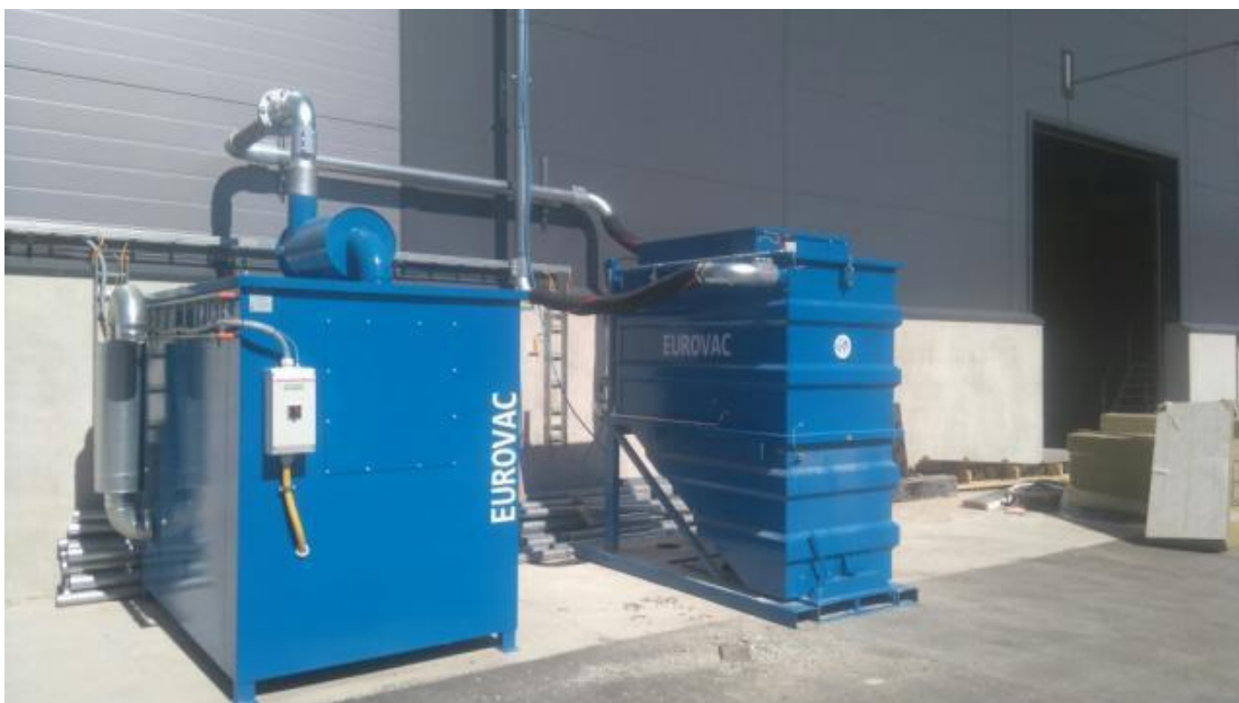
Eurovac 45 kW rootspump + filtercontainer
