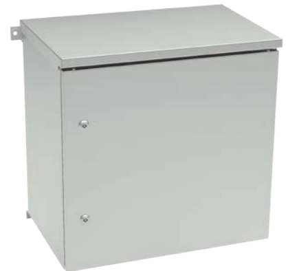
SWN IP65 cabinet with mounting plate and 19" rack, powder painted in RAL 7035 (light grey). External dimensions: height 575 mm, width 600 mm, depth 400 mm. Usable height 12 U. Versions with solid and glazed doors.
