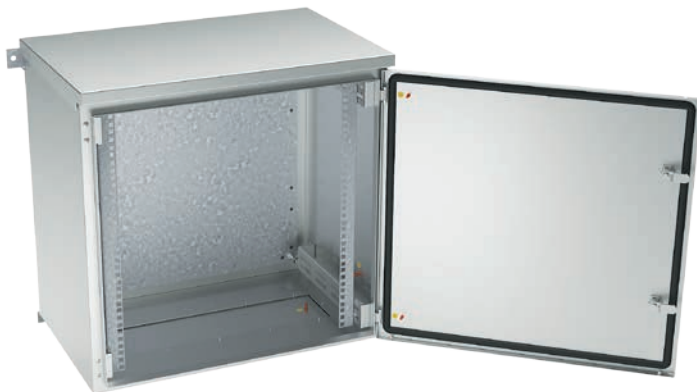
SWN Inox IP65 cabinet with mounting plate, 19" rack and rain hood. External dimensions: height (with hood) 606 mm, width 600 mm, depth 400 mm. Usable height 12 U
