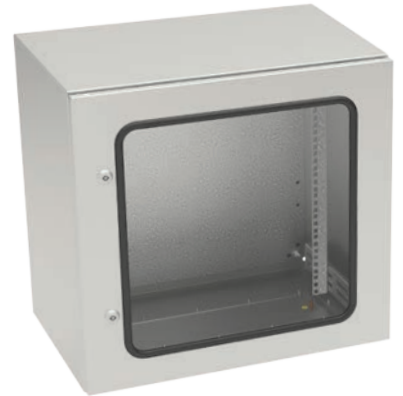
SWN IP65 cabinet with mounting plate and 19" rack, powder painted in RAL 7035 (light grey). External dimensions: height 575 mm, width 600 mm, depth 400 mm. Usable height 12 U. Versions with solid and glazed doors.
