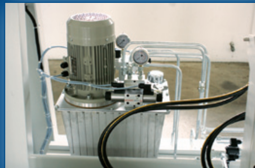
Central hydraulic unit
