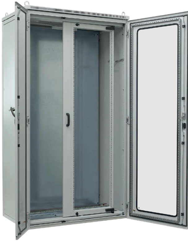
1200 mm wide SZE2 cabinet with mounting plate, swing frame and asymmetrical double-leaf door
