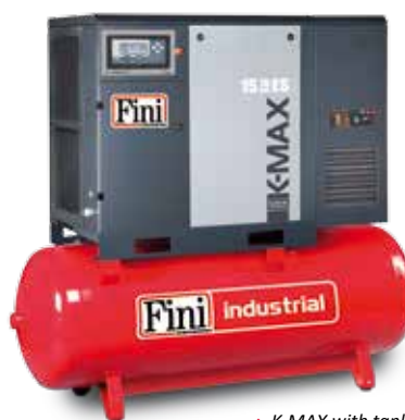
▲ K-MAX with tank and dryer
