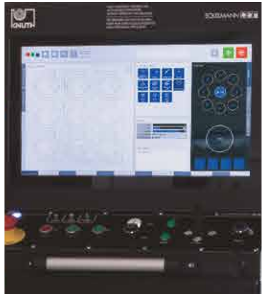
Eckelmann CNC unit with 19" touchscreen for TrueCut K models
