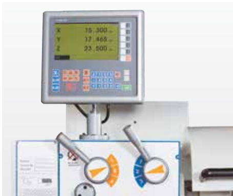
Positioning indicator on X, Z and Z1 axis
