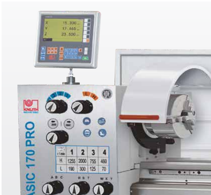
Position indicator on X-, Z- and Z1-axis
