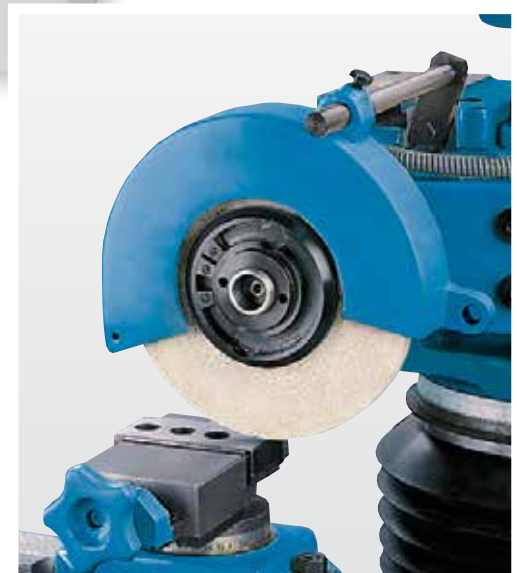
Surface grinding with angle-adjustable vise
