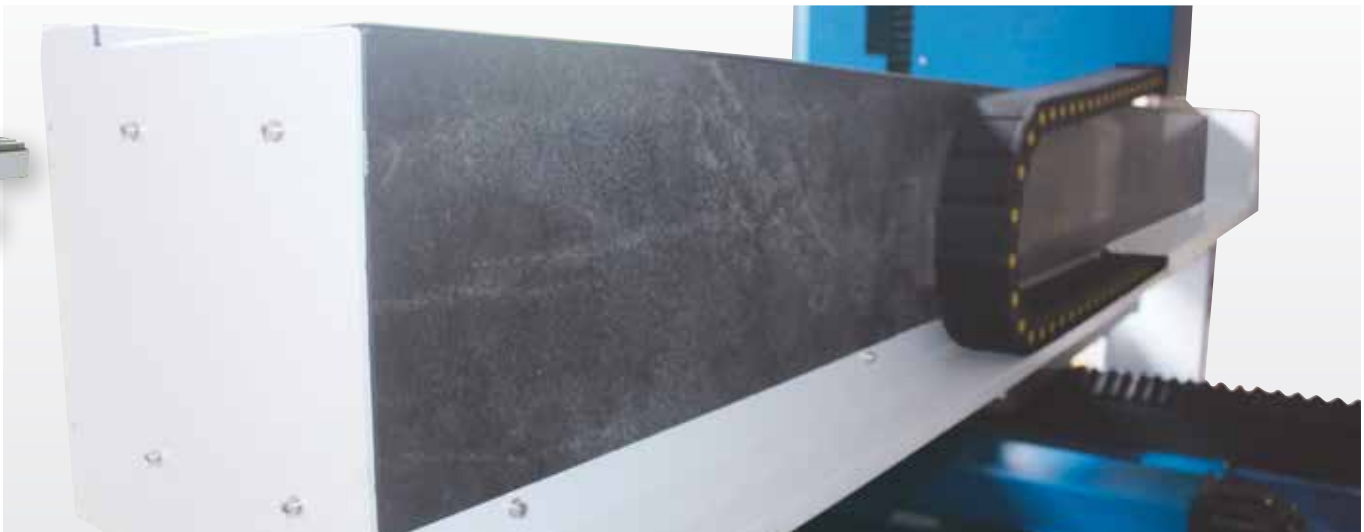
Precision-ground granite elements on all axes
