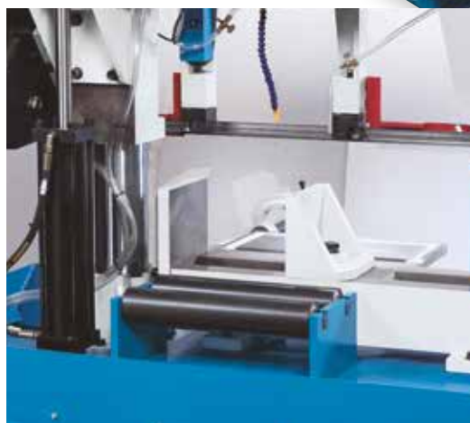
Roller support for easy material advancement
