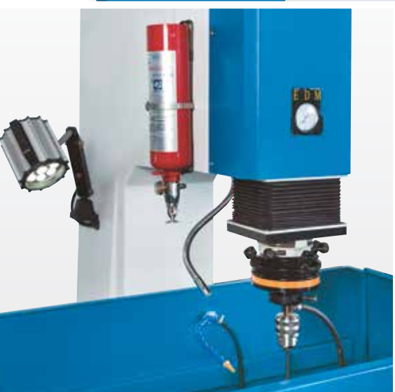
Fire extinguishing system for added safety
