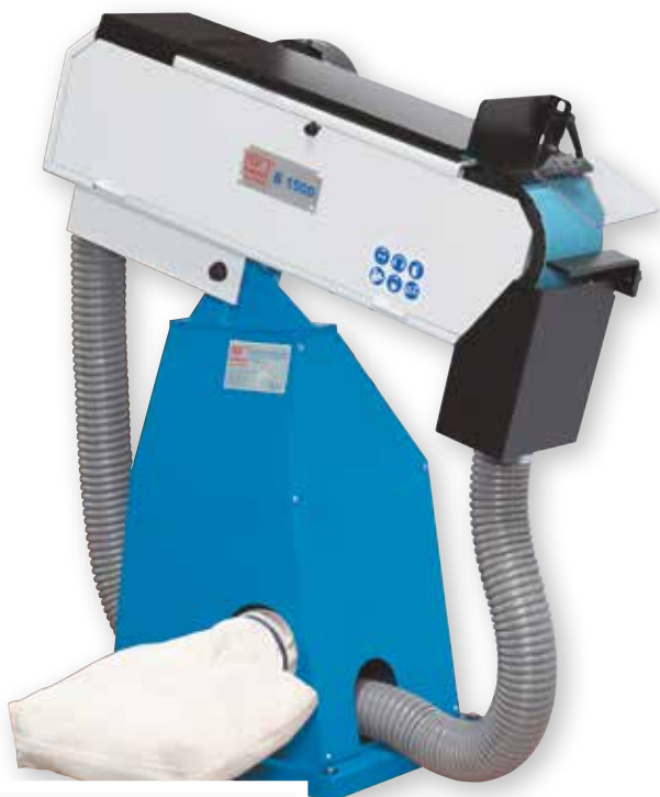
Fig. B 150 D with integrated suction
