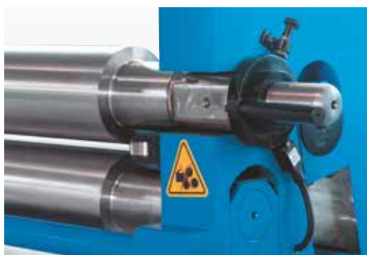
Upper roller can be swiveled out
