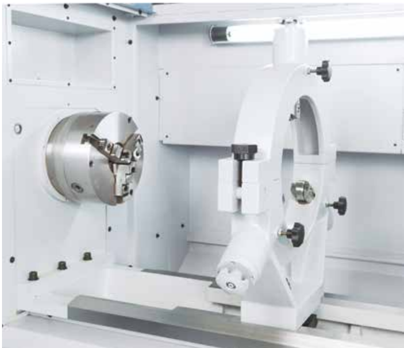
Option: steady rests up to 400 mm diameter
