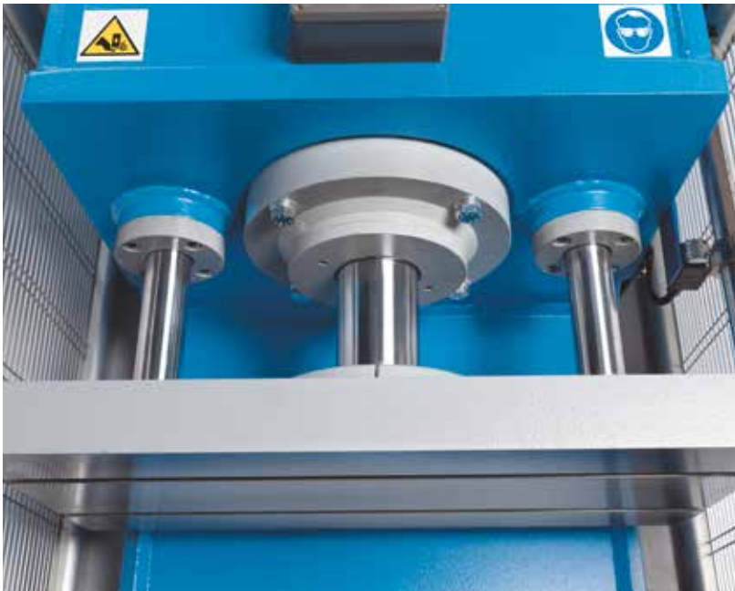
Two circular guides ensure maximum ram plate parallelism during stroke movement
