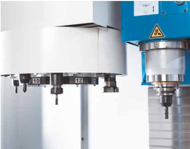
Rugged horizontal tool changer with 12 stations
