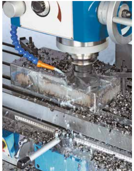
Face milling with cutter head
