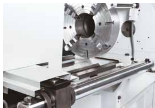
Taper turning unit is included
