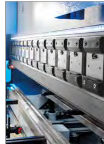
PROMECAM Mechanical Clamping
