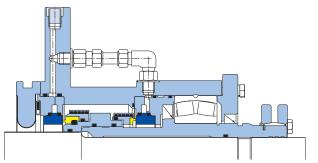
Mixmaster VII-DD™ - Inboard and outboard cooled stationary seat option
