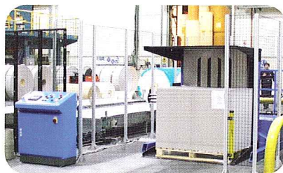
PT1500APA - Automatic pile turner with max. format 1040 x 1440 mm installed at a paper converting company.
