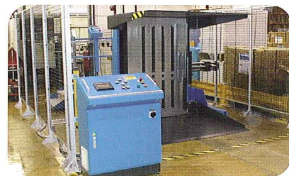
PT1800APA - Automatic pile turner with max. format 1200 x 1600 mm installed at a display-printing company.
