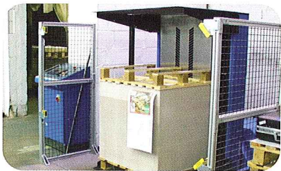
PT1000APA - Automatic pile turner with max. format 740 x 1040 mm installed at a commercial printing company.
