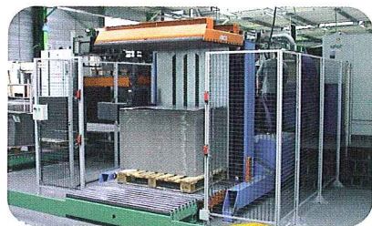
PT2500APA - Automatic, front loaded pile turner for max. sheet format 1200 x 1450 mm installed in a packaging production line.
