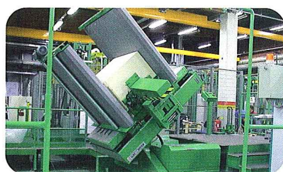
PT2500APA - Automatic, side loaded pile turner for max. sheet format 1450 x 1600 mm installed in a paper mill packaging line.
