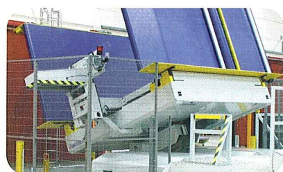
PT3500APA - Automatic, side loaded pile turner for max. sheet format 1600 x 3300 mm installed at a packaging company for aerating, jogging and aligning of fluted board.
