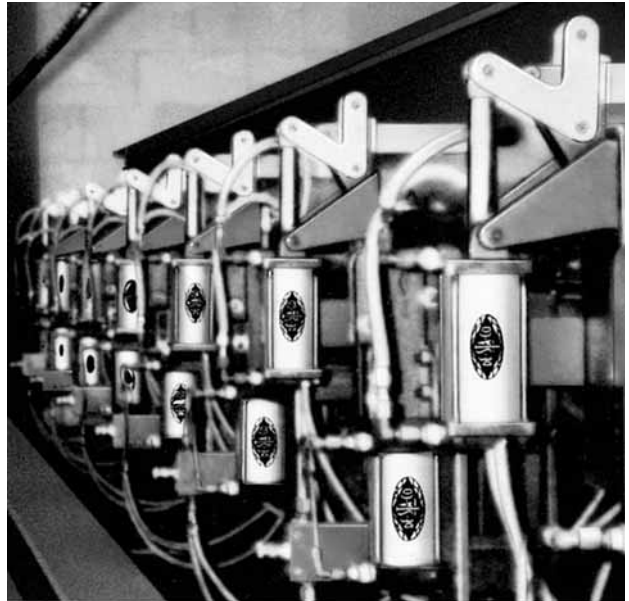
Power clamp model 868 in an automated welding fixture for clamping of longitudinal beams.
