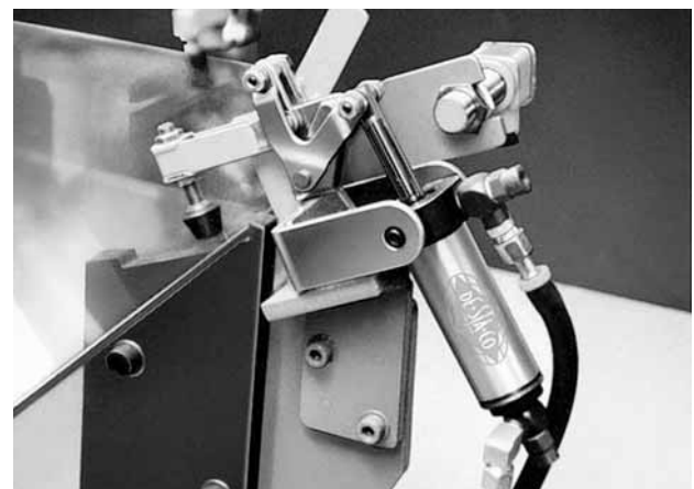
Power clamp model 817-UF on a pneumatic clamping fixture
