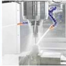
Spindle ring form coolant cooling is fast. Ability of chip conveyor is strong. More suitable for thin hole machining
