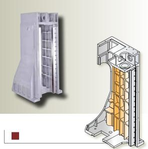
The column is made of high grade dense cast iron which has been stress relieved. With ribbed and computer-analyzed structure, the stability and rigidity is greatly increased. Spindle travels on hardend and ground square ways, and is driven by precision ballscrew and an AC servo motor for heavy grinding and smooth & accurate movement.
