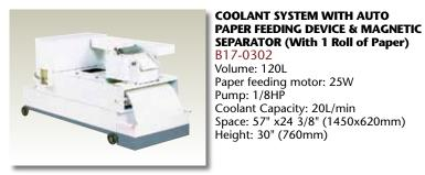
**SEPARATOR (With 1 Roll of Paper)** B17-0302 Volume: 120L Paper feeding motor: 25W Pump: 1/8HP Coolant Capacity: 20L/min Space: 57" x24 3/8" (1450x620mm) Height: 30" (760mm)
