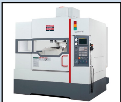
MV184 , kraftfull vertikal flerop, XYZ = 1020x610x610.
