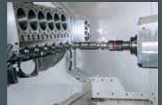
Pump bore in a truck motor block: diameter & concentricity
