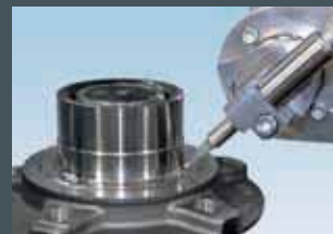
Crack Detection Testing Machines (eddy current)
